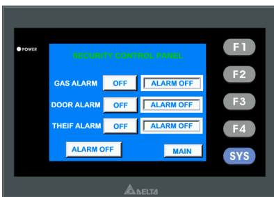
Figure 11 Security control panel
