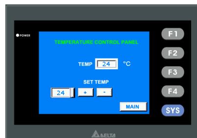
Figure 12 Temperature control panel
