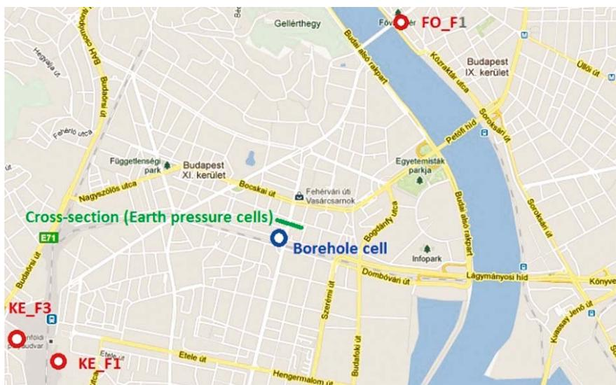
Figure 1. Measurement points (Selfboring Pressuremeter: FO\_F1, KE\_F1, KE\_F3; Borehole cells and Earth pressure cells)
