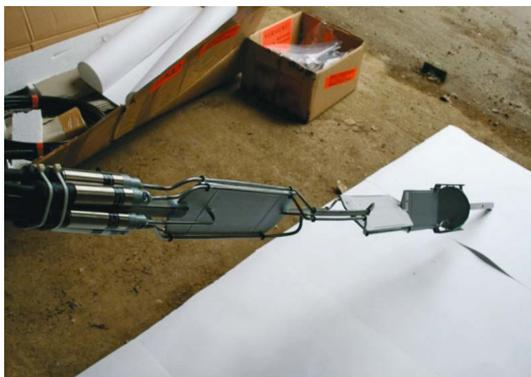
Figure 3. Borehole cell (Glötzl Ltd).
