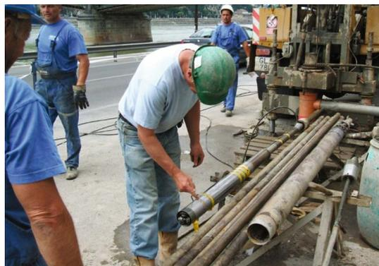
Figure 4. Selfboring pressuremeter
