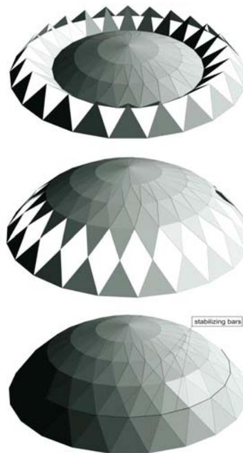
Figure 4 Schema of the of the pantadome erection
