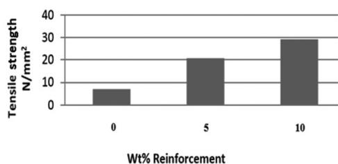
Fig. 3 Tensile strength vs wt % of SiO<sub>2</sub>
