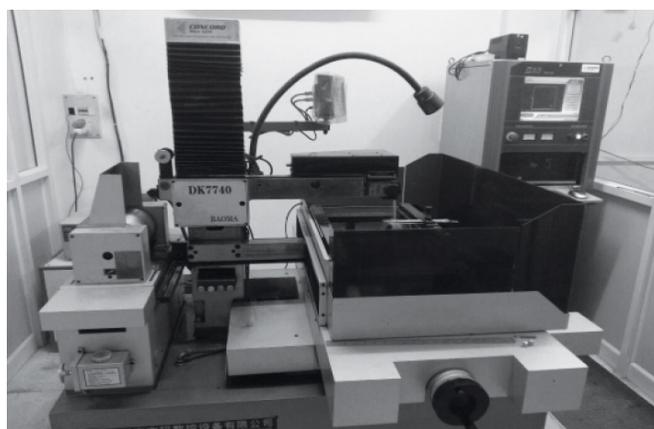
Fig. 7 Wire cut EDM machine
