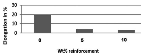
Fig. 6 Elongation vs wt % of SiO<sub>2</sub>
