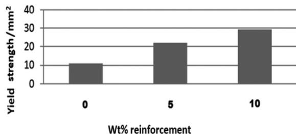
Fig. 5 Yield strength vs wt % of SiO<sub>2</sub>
