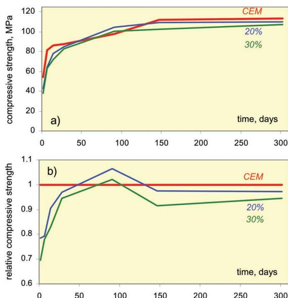
Fig. 7. Compressive strength and relative compressive strength of specimens with green WGP
