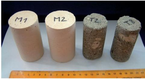
Fig. 1. Cylindrical coarse limestone and rhyolite tuff specimens
