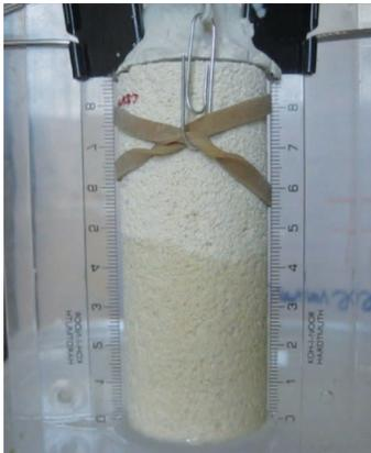
Fig. 1. Testing setup for the capillary elevation measurement
