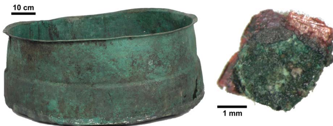
Fig. 6.: Late Roman copper cauldron (photo: A. Dabasi, Hungarian National Museum) and one of the corroded metal samples taken from the cauldron.
