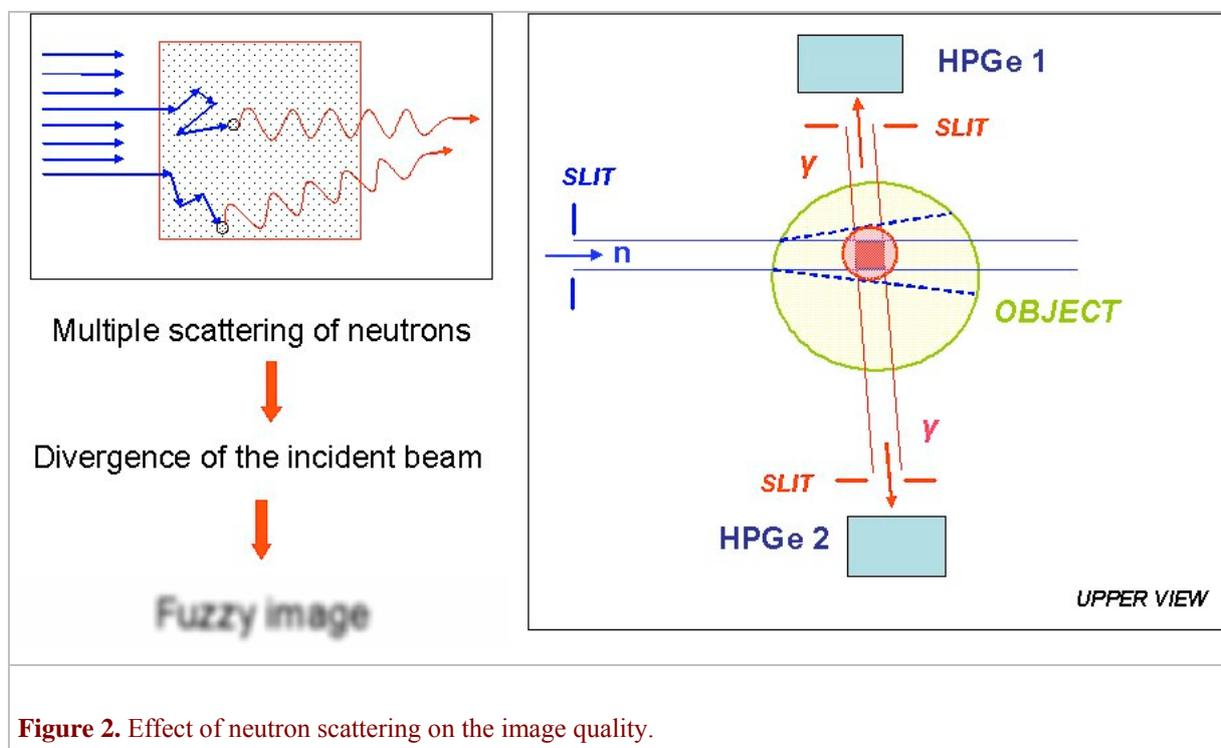
**Figure 2.** Effect of neutron scattering on the image quality.
