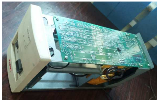
Figure 6 An uninterruptible power supply as a DC/AC converter
